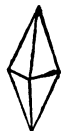
Fig. 178. The pyramidal octohedron, with scalene, triangular faces. This is the primitive form.
